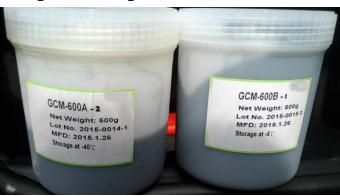
An protective ink sets as G2 overcoat in chip resistor. This ink gives excellent printing and moisture resistance.
